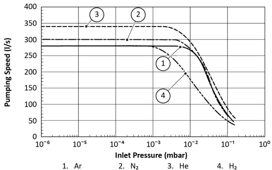
**Figure 4** nEXT400 performance curve
