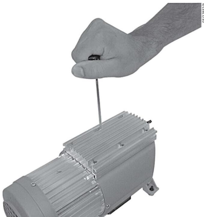
9. Assemble handle with screws and tighten.
