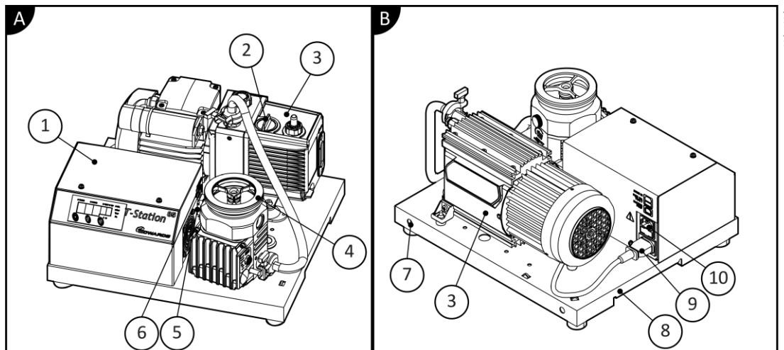
A. Front view (T-Station with E2M1.5 backing pump option)
