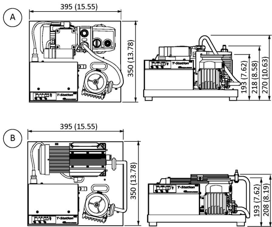
A. T-Station 85H wet with E2M1.5 backing pump
