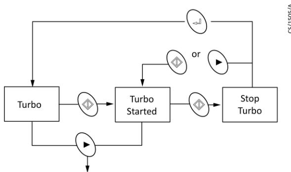
**Start the pump with the turbo screen**
