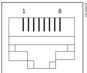
**Table 7** Active gauge connector pin-out
