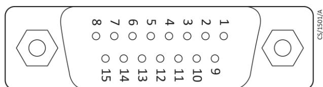
**Table 6 Turbo pump connector pin-out**
