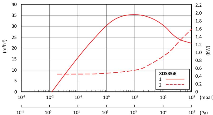
The power consumption of the enhanced version at high inlet pressure can be lowered by a further 100 W more with the installation of a second exhaust silencer by an NW25 T-piece.
