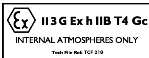
This equipment is intended to be installed in a safe non-hazardous area and its design meets the requirements of Group II Category 3 equipment in accordance with EU and UK Legislations concerning equipment and protective systems intended for use in potentially explosive atmospheres.
