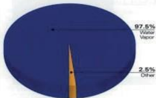
Water vapor comprises over 97% of the residual gas load at 10^{-3} Torr and below
