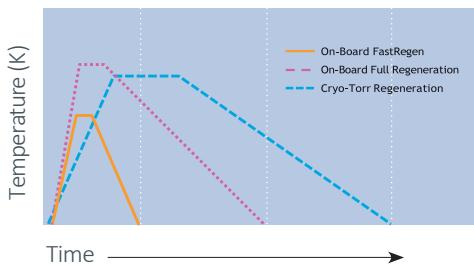
Moreover, On-Board’s FastRegen® capability further increases uptime by swiftly removing only the process gasses, restoring its performance in a fraction of the time required by a full regeneration.
