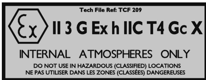
This equipment is designed to meet the requirements of Group II Category 3G in respects to ignition sources internal to the pump. This classification is in accordance with Directive 2014/34/EU.
