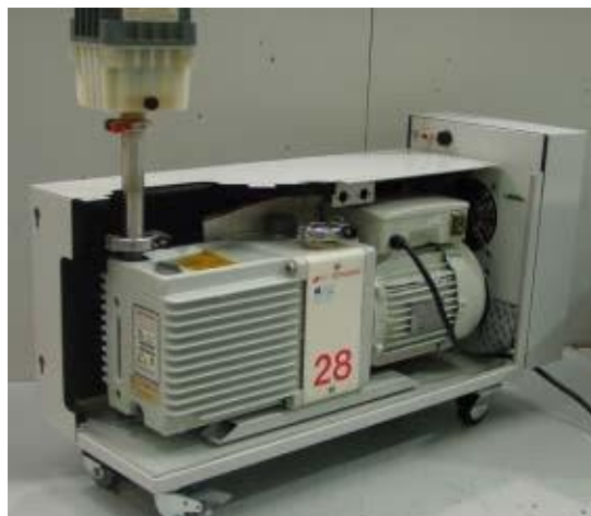
Figure 10 - Removing panel to gain access to filler cap
