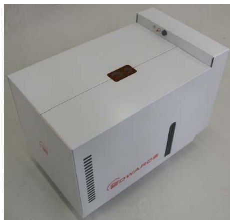
Figure 4 - Fitting second cover to right hand side of pump
